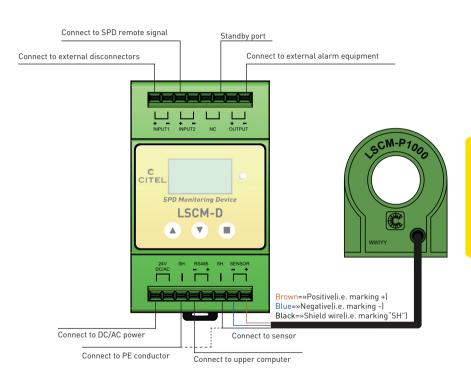
Fig3. Typical LSCM-D wiring connection
