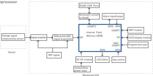
Fig1. LSCM-D system schematic diagram
