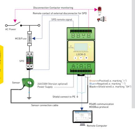
Fig4. Typical wiring diagram for LSCM-D
