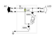
V: Varistor GSG: Specific gas tube LED: Disconnection indicator Ft: Thermal fuse
