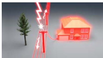
3. Strike on overhead lines
