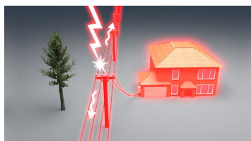
3. Strike on overhead lines
