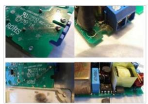
Examples of destruction to LED arrays and drivers due to lightning surges
