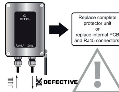
Replace complete protector unit or replace internal PCB and RJ45 connectors.
