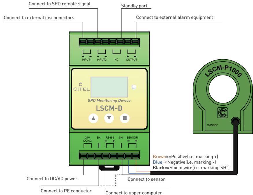
Fig3. Typical LSCM-D wiring connection
