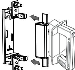
The fuse linkwith the replacement handle is inserted into the fuse base to the end.
