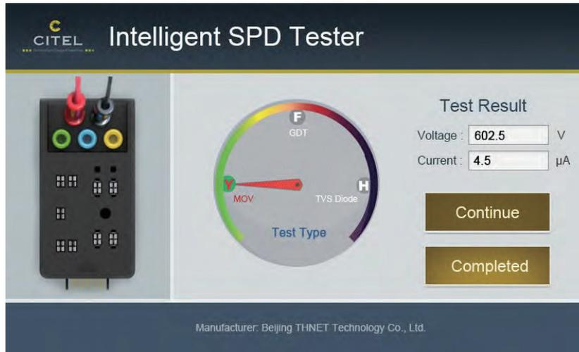
**Figure 5-14** Display of the test result for a manual test type
