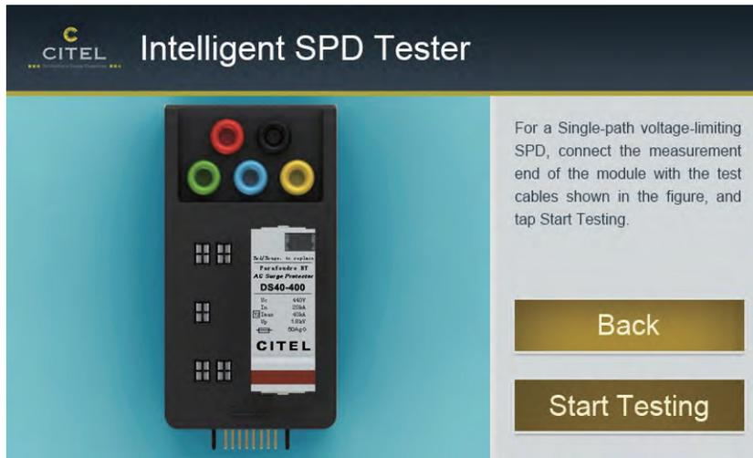
Figure 5-6 Testing a plug-in module
