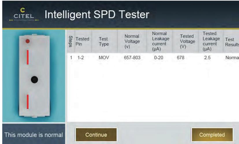
**Figure 5-9 Screen displayed after the test is completed**
