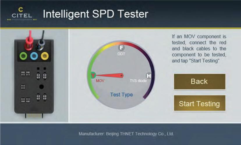
Figure 5-12 Display of the screen for confirming the manual test type
