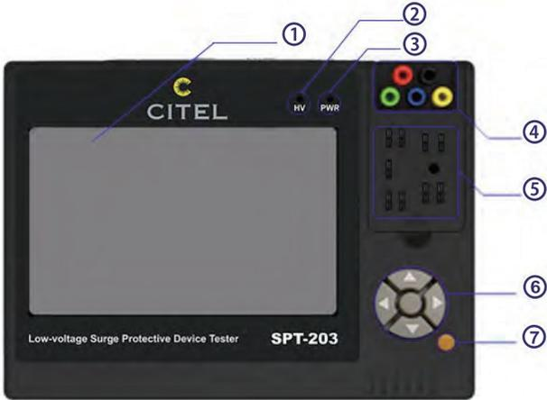
Figure 2-2 Front view of the tester
